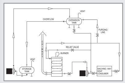
It has a three-pass combustion chamber which utilizes maximum heat of the flue gases and hence makes the unit cost-effective.
