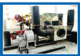
SI Series Medical Incinerator is a useful type waste disposal equipment Which can be used in every class hospital for incinerating solid flammable waste such as surgical waste and substance with virus etc.
